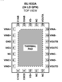
pin-to-pin drop-in compatibility with the EL1528. The ISL1532A integrates 50k pull-up resistors on  $\rm C_{\rm O}$  and  $\rm C_{\rm 1}$  pins.
